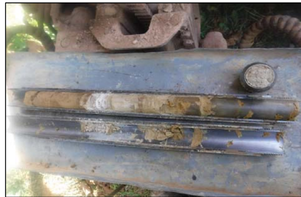
Foto 6: S-1; SPT a 9,0 metros
