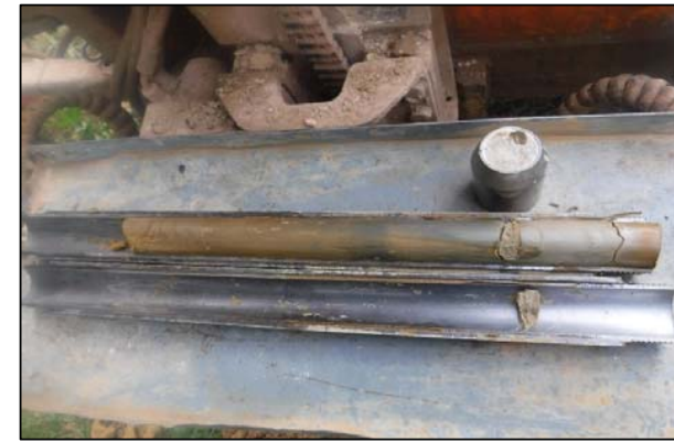
Foto 7: S-1; SPT a 12,0 metros
